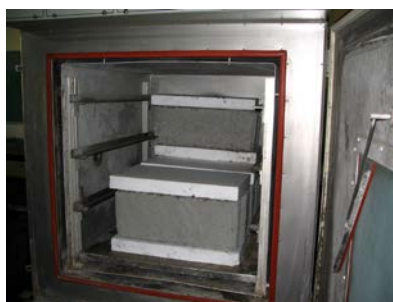
(b) Negovanje u termo-komori Curing in the thermo-chamber
